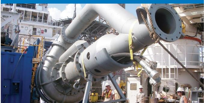
The **Toyo submersible DP series** and its hydraulically driven cousin the **TO series** were specifically designed to pick up and transport abrasive materials with the least amount of water.
