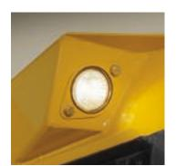
High-intensity halogen driving lights are standard. Or opt for the factory-installed 360-degree light package and extend your workday beyond normal daylight hours.
