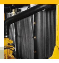
No stacked coolers in these crawlers. Side-by-side cores with wide fin spacing reduce clogging and are easy to clean.
