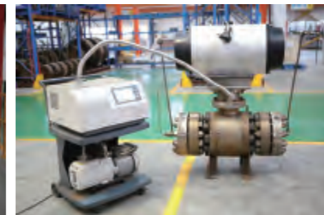
Low Fugitive Emission Test
