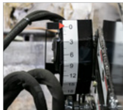
Depth indicator makes it easy to know depth of cut being made.
