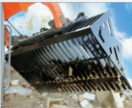
Grade 80 steel tine material with front gusseted tine tips.
