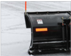
Radiused blade rolls snow more efficiently, while providing 30° of angle.
